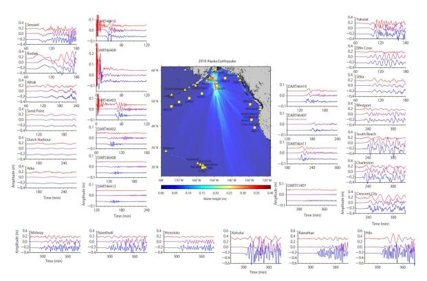
Figure 2. Simulated maximum tsunami height for the 2018 Alaska earthquake and comparisons of tsunami waveforms. Solid lines in red and blue indicate the observed tsunami waveforms and calculated ones, respectively. Purple lines show the phase-corrected tsunami waveforms.
