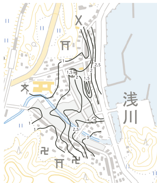
Fig.17 Height of flooding from the ground
