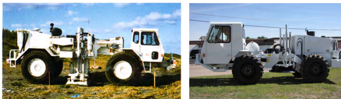
Fig. 6-12 Photos of Seismic vibrators (Vibroseis) for PS logging and VSP survey
