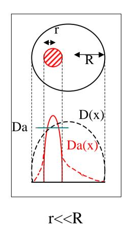
$\Delta \sigma$  for single asperity (=9.5MPa) =  $\Delta \sigma$  for single crack (=9.6MPa)
